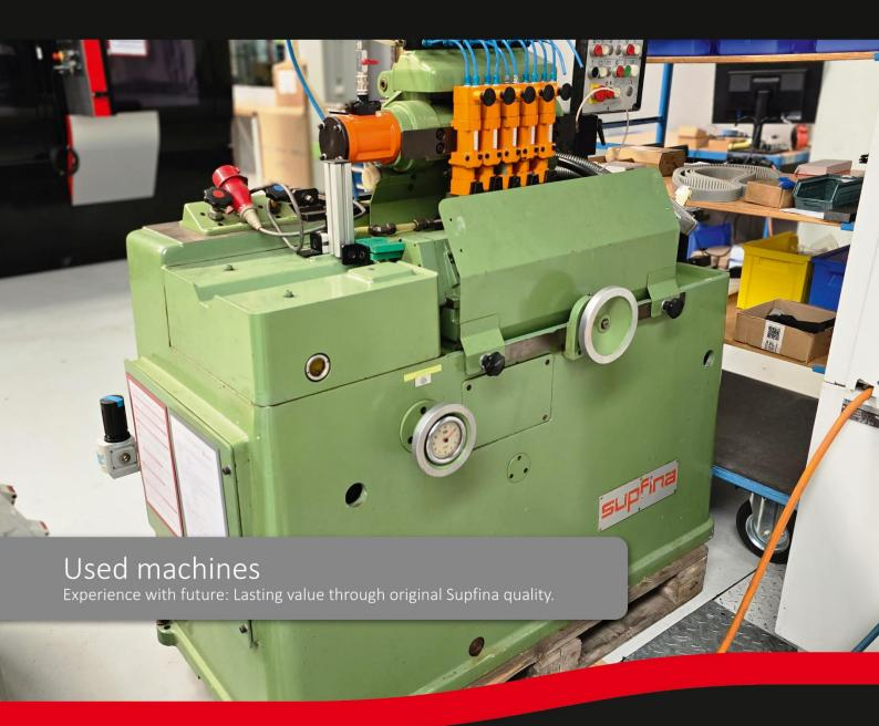
Superfinishing machine for through feed grinding
