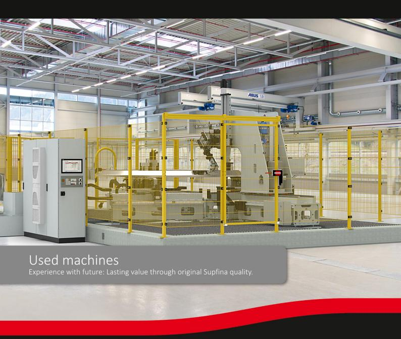
Superfinishing machine Machining of cylindrical and tapered roller bearings, Inner and outer rings
