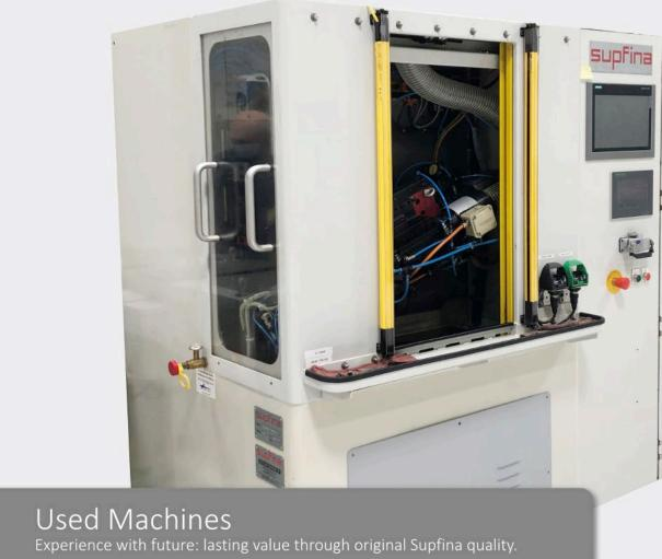
Compact Superfinishing machine for flat finishing
