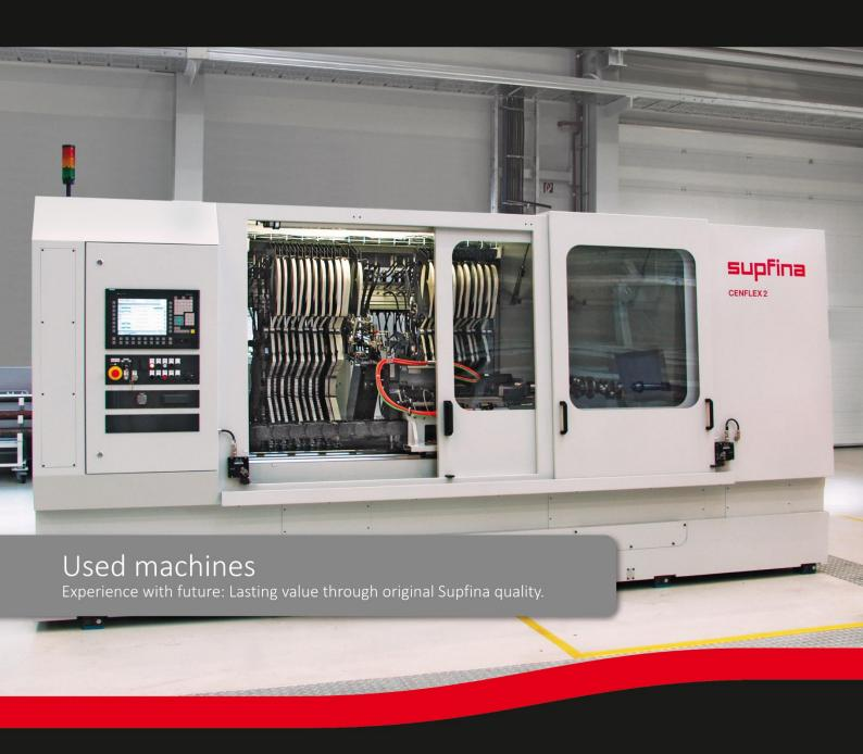
Superfinishing of crankshafts and camshafts
