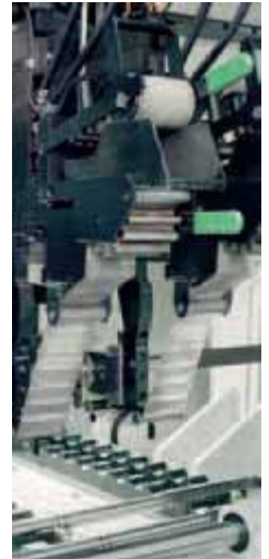
The advancement of the tape after every machining cycle guarantees consistent results
