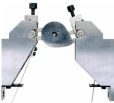
Stone machining of cams using specially developed oscillating stone holders for the prevention of profile deformations.
