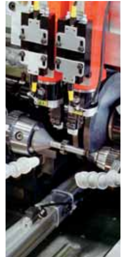
Machining procedure for a pump pinion Machining of bearings and faces
