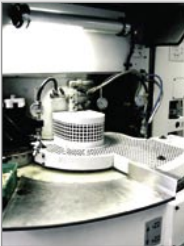
Manual insertion of the parts into the transport disk
